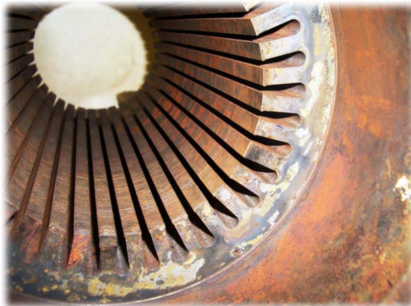
Figure 2: Stator Processed in a Burnout Oven
