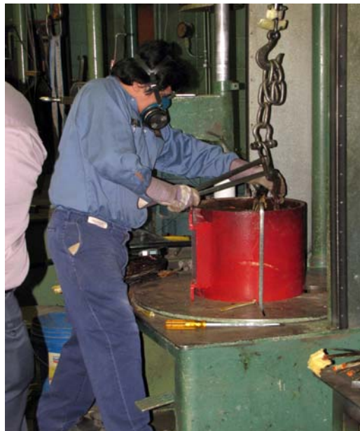
Figure 1: Mechanical Stripping Stator
