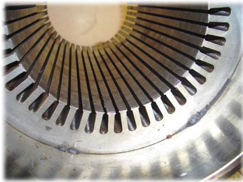
Figure 3: Stator Processed with Mechanical Stripping
