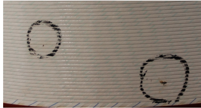
Fig 3: Burn Spots Between Primary Conductors
